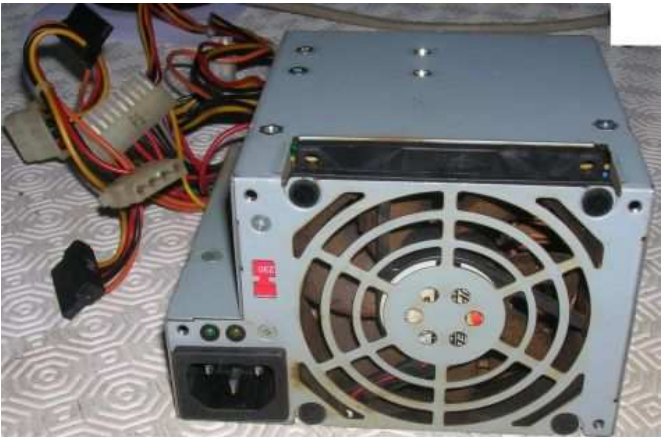
Alimentatore API4PC51 P/N: 24R2585 CRU: 24R2584 EC: H18532 REV.: D AC INPUT 100-127V 50/60hZ, 6.0A 200-240V 50/60hZ, 3.0A TOTAL POWER 225W MAX
