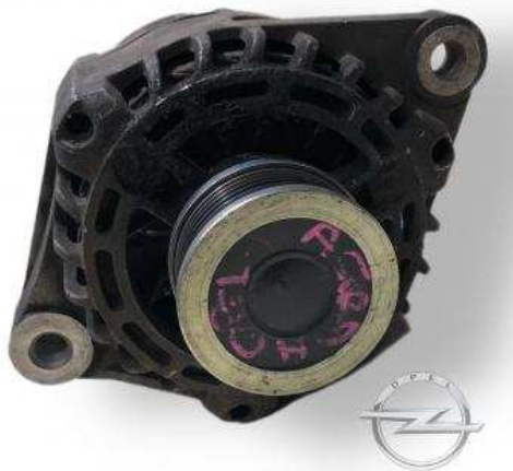
Alternatore 1.9 CDTI OPEL ASTRA VECTRA SIGNUM ZAFIRA DENSO MS1022118641, YM 13117340, 105A
